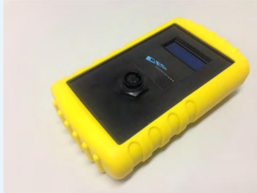
Readout can be made using Geosystems low cost manual readout box, which performs diagnostics on the lead-wires, recognizes the sensor type and ID and outputs the displacement and temperature data directly in mm and °C.
