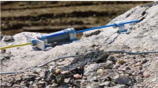
Geosystems **digi-Crackmeter** displacement sensor integrates magnetostrictive technology to produce a high precision digital instrument comprising a non-contact displacement sensor and digital temperature sensor. An on-board microcontroller applies temperature compensation and outputs a digital signal. Both the resolution (<0.01mm) and accuracy (0.25% linearity typical) are significantly better than for similarly priced technology.
